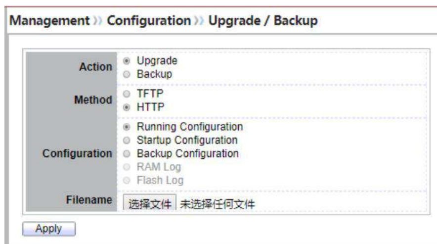
Figure 14-8 Upgrade Configuration through HTTP
