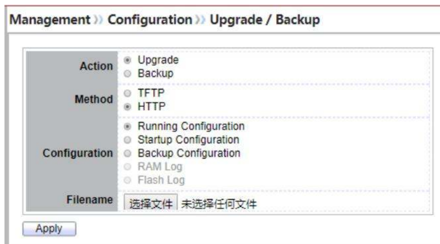
Figure 14-8 Upgrade Configuration through HTTP
