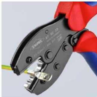
Figure 7 Crimping the Ring Terminal
