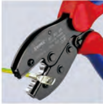
Figure: Crimping the Ring Terminal
