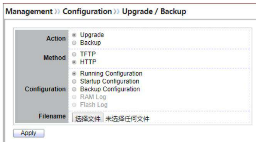
Figure 14-8 Upgrade Configuration through HTTP
